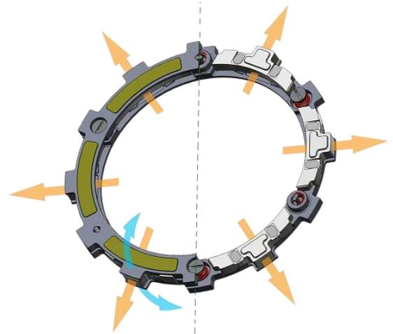
**RPM Increases > Wedges Slide Out > EXP Disk Expands > Clutch Engages**
